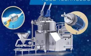
Gold Peg's latest creations, the ShearTherm (above) and FreeTherm batch cooking systems offer companies cuttingedge technology to help grow their business. The ShearTherm is purposedesigned with high shear mixing flexibility for the likes of high powder content recipes to achieve homogeneous, fully hydrated, blended and cooked product. The multi-functional, cost-effective FreeTherm is designed to blend, cook and de-aerate a wide range of food products.
